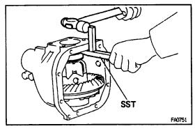
(c) Using SST and a hammer, remove the 2 side plate washers.
