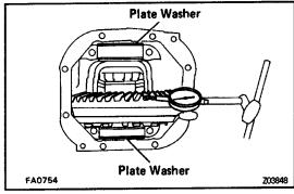
(k) If the backlash is not within specification, adjust by either increasing or decreasing the number of washers on both sides by an equal amount.
