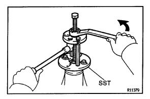
(c) Using SST, remove the companion flange. SST 09950–30010
