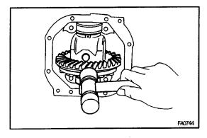
(b) Tap on the ring gear with a plastic–faced hammer so that the washer fit to the bearing.
