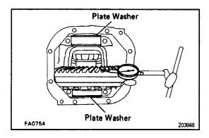
(e) If not within specification, adjust by either increasing or decreasing the washers on both sides by an equal amount.
