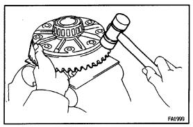
(d) Using a plastic–faced hammer, tap on the ring gear to separate it from the differential case.
