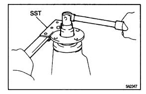
(d) Adjust the drive pinion preload by tightening the companion flange nut.
