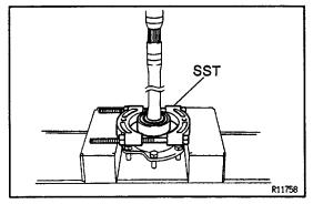
(b) Using SST and a press, remove the bearing. SST 09950–00020
