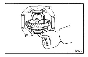
(d) Using the backlash as reference, select a ring gear back side plate washer. (See page SA-98)
