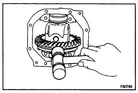
(i) Tap on the ring gear with a plastic–faced hammer so that the washer fit to the bearing.
