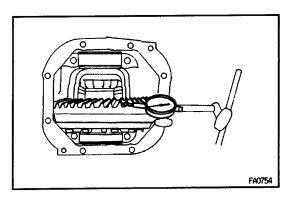
(j) Using a dial indicator, measure the ring gear backlash. **Backlash:**
