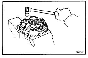
(c) Remove the 10 bolts and 5 lock plates.
