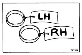
(d) Remove the differential case with the bearing outer races from the differential carrier.
