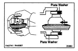
(h) Place the other plate washer onto the differential case together with the outer race, and install the differential case with the outer race into the carrier.
