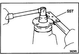
(b) Using SST to hold the flange, remove the nut and plate washer.
