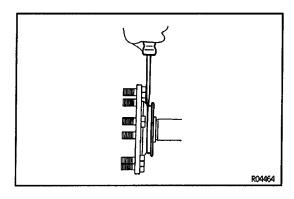
(c) Using a screwdriver and hammer, remove the dust cover.
