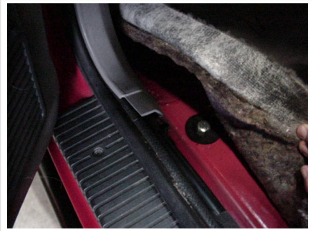
Figure 10 , Front floor hole under carpet.
