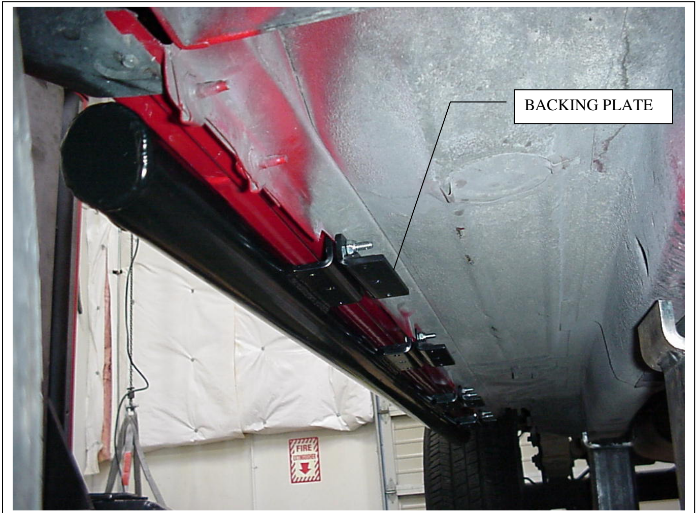
Figure 7, Rock Slider installed with backing plates.
